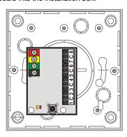
Wired loops are wired to inputs 1 to 8 with the C terminals as the common line.
