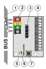
Fig 2: 1 – BUS cable; 2 – BUS terminals; 3 – production code (on the bottom of the PCB); 4 – input terminals for external magnetic detectors; 5 – yellow LED; 6 – red LED; 7 – tamper contact
