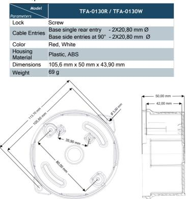
The deep base is suitable for use with any base having an 80 mm fixing
