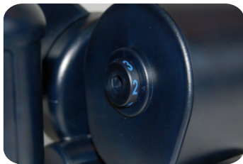
Diaphragm position 2 Distance from 30 m up to 90 m
