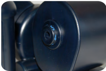
Diaphragm position 4 Distance from 15 m up to 120 m
