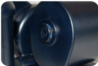
Diaphragm position 4 Distance from 15 m up to 65 m
