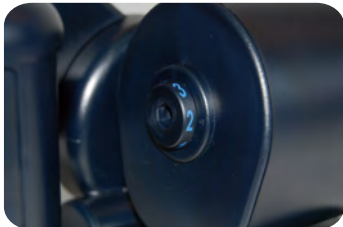
Diaphragm position 2 distance from 40 m to 170 m
