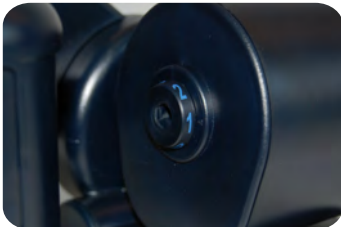
Diaphragm position 1 distance from 50 m to 180 m
