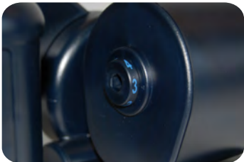
Diaphragm position 3 distance from 30 m to 150 m
