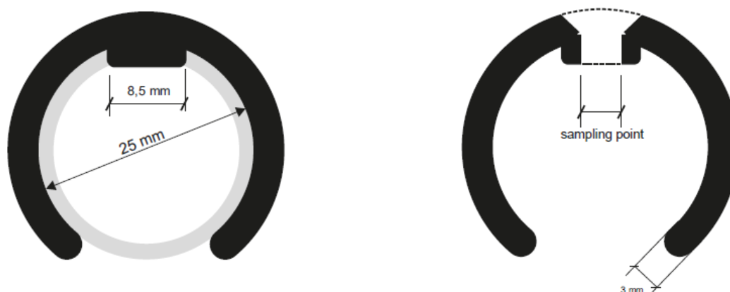
Fig. 3 Drawing sampling clip / maintenance clip PA
