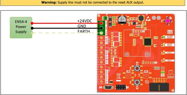
Figure 4 – Supply Connection Diagram
