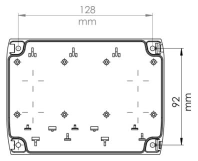
Figure 1 – Mounting Hole Sizes
