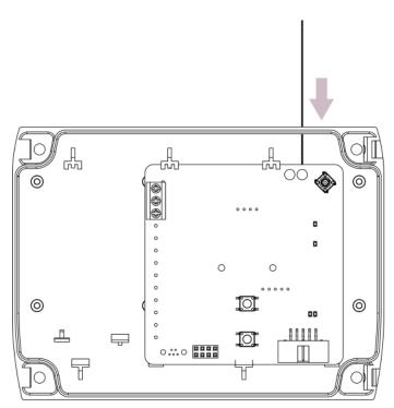
Figure 2 – Antenna Wire Installation
