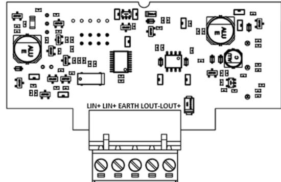
3. EARTH connection must be connected both on control panel and inside of manual call point to ensure integrity
