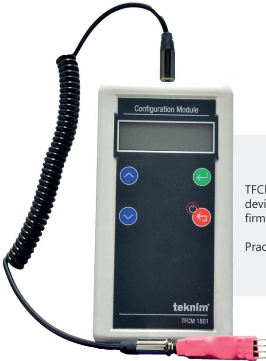
TFCM-1801 device programming module is developed to define address for addressable devices such as detectors, mcp, input-output modules or to read defined address and firmware version of the devices. It is supplied from 9V (6LR61) battery.
