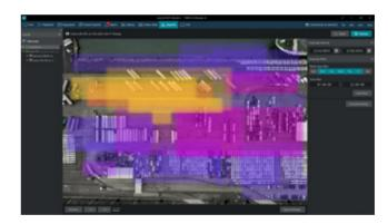
The Heat Map tab in the Monitor application outlines motion intensity by colour based on accumulated VCA data.
